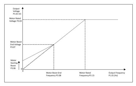
For Linear V to F, the voltage to frequency characteristic can be adjusted at two points, 0 Hz where the starting boost voltage is set in *Motor Starting Boost* (P3.06), and *Motor Starting Boost End Frequency* (P3.08), *Motor Starting Boost End Voltage* (P3.07) which is the frequency and voltage point at which the boost level is tapered to.
