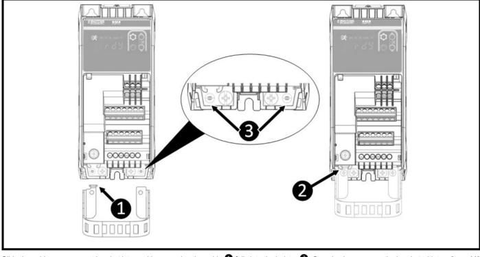
Slide the cable management bracket into position ensuring the guide **1** falls into the holster **2**. Once in place, secure the bracket with two 6 mm M3 screws (supplied with accessory) into holes **3** with a phillips or 3 mm (1/8 in) slotted screwdriver. The screws should be tightened with a maximum torque of 1.5 Nm (13.27 lb in).
