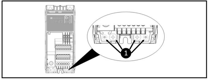
The ground loop impedance must conform to the requirements of local safety regulations. The drive must be grounded by a connection capable of carrying the prospective fault current until the protective device (fuse, MCB) disconnects the A.C. supply. The ground connections must be inspected and tested at appropriate intervals.
