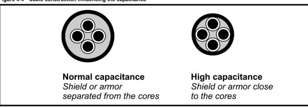
Figure 4-4 Cable construction influencing the capacitance
