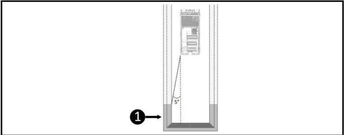
Openings for cables etc. must be sealed with materials meeting the 5VB requirement, or else have a baffle above. See Figure 3-2 for acceptable baffle construction. The distance below the drive where this applies to the enclosure wall = Distance from the cabinet wall to the drive  $\div$  0.0875.
